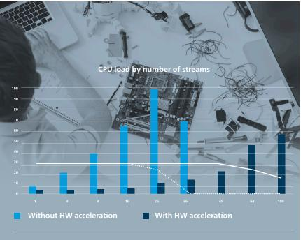
XProtect Smart Client performance measured for h.264 stream format displayed in full HD. Tested hardware: Windows PC with Intel Core i7-8700K processor at 3.70GHz, 32 GB RAM, 2X NVIDIA GeForce GTX 1080 8GB
